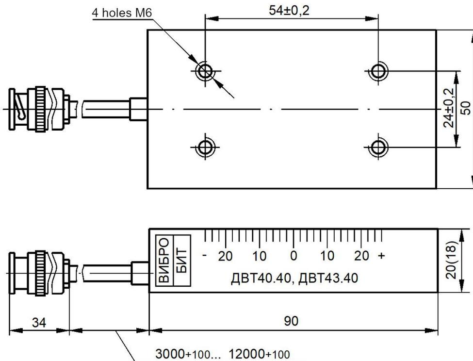
Figure C.7 - Sensors ДВТ40.40, ДВТ43.40
