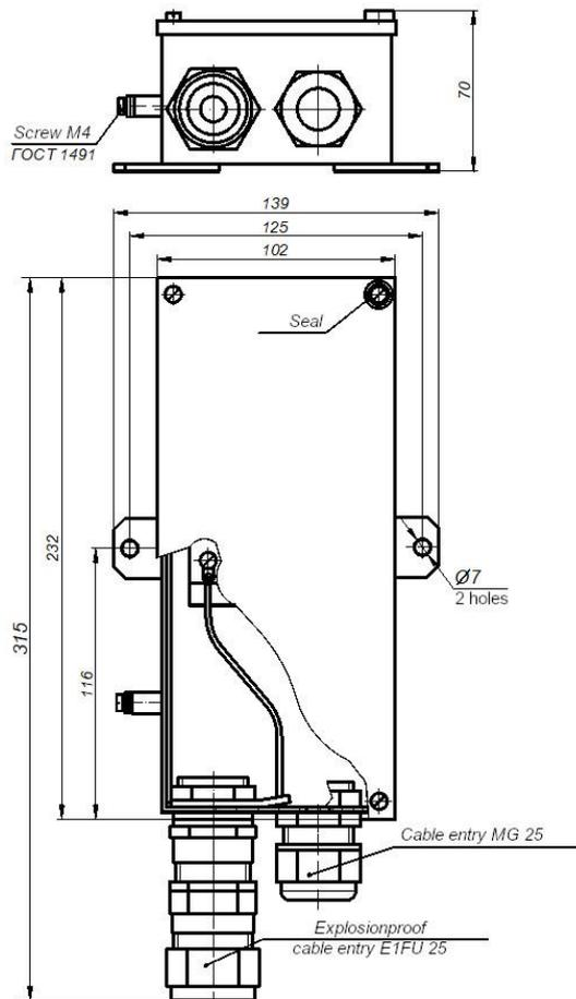
Figure C.39 – Transducer box КП13Х
