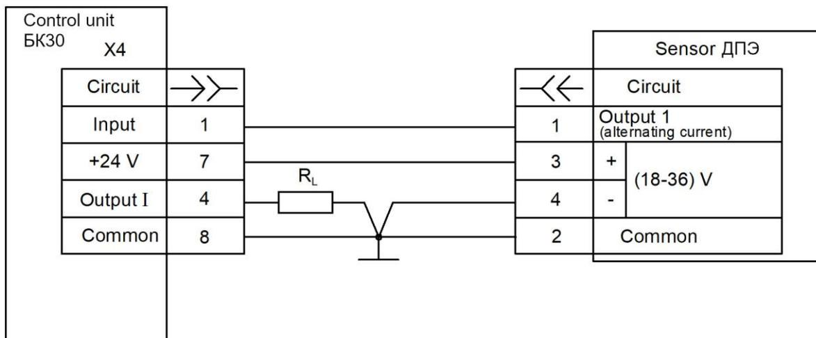
$R_L$  – unified signal load resistance.
