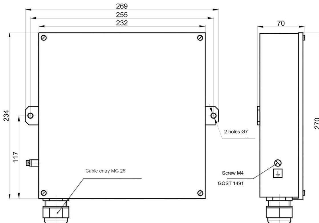
Figure C.34 – Transducer box КП23П
