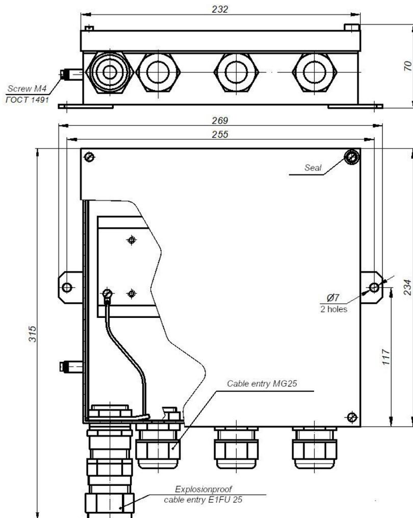
Figure C.33 – Transducer box КП23ВХ
