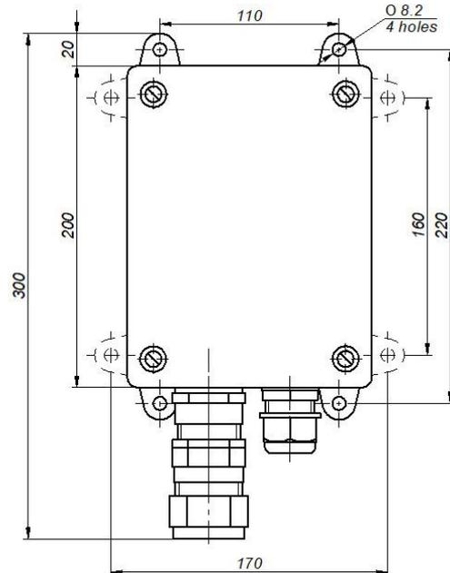
Figure C.41 – Transducer box КП13XP
