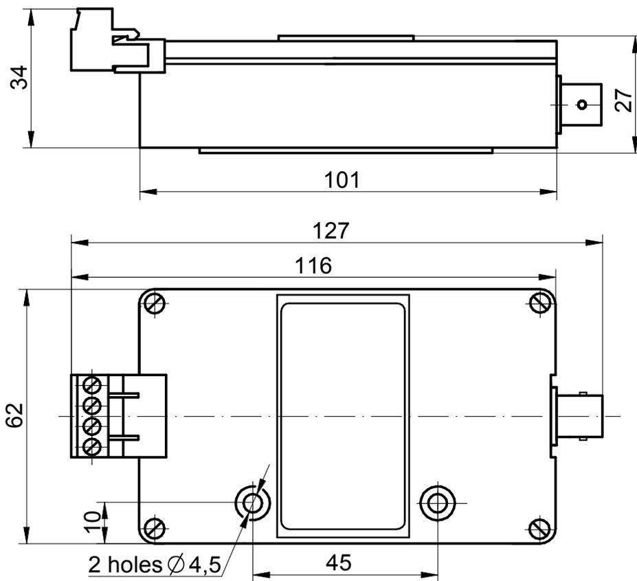
\* - ИП34 converter is available with two types of connectors:
