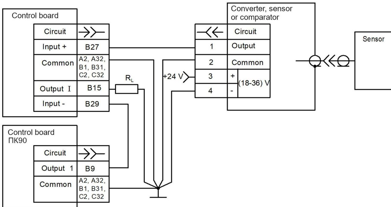
$R_L$  – unified signal load resistance.
