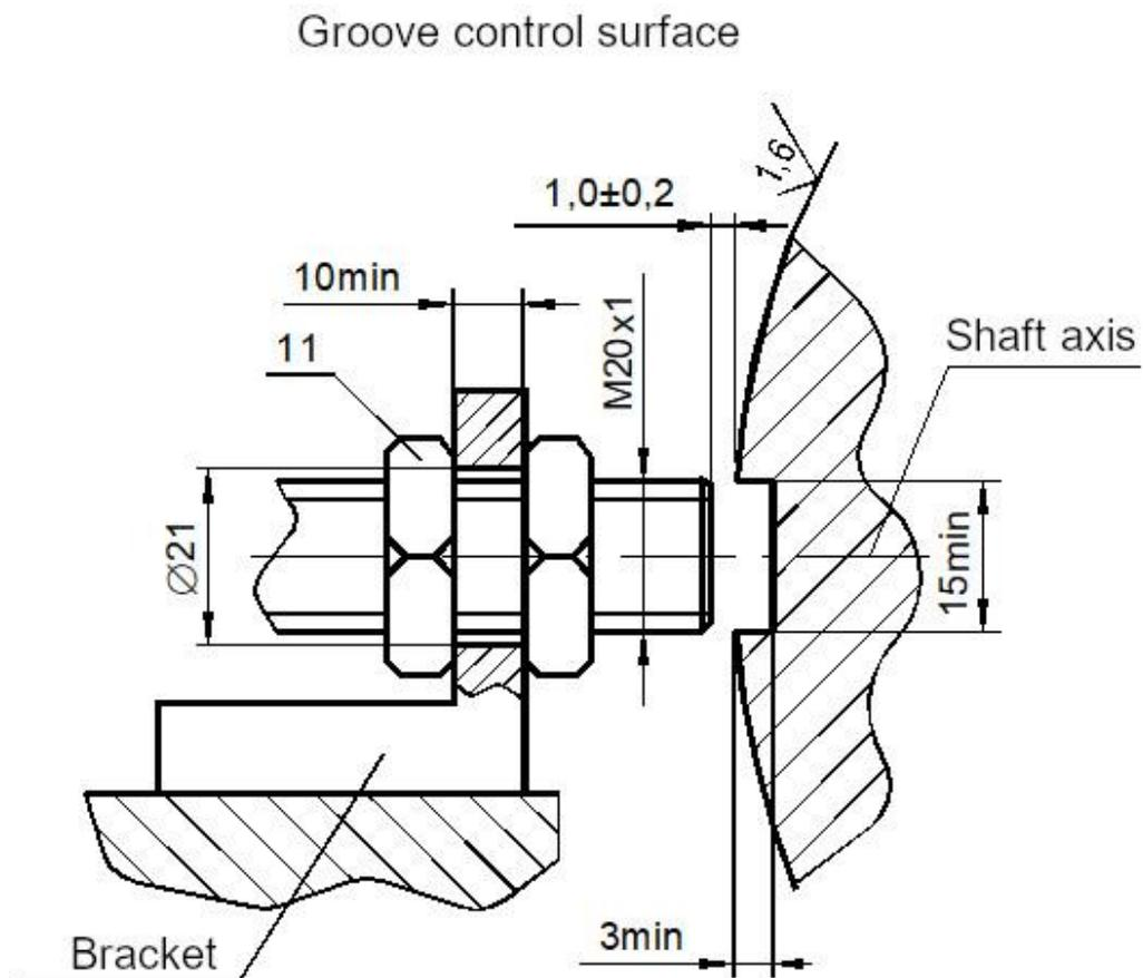
Note – For sensor ДХМ – preset gap – from 1 mm
