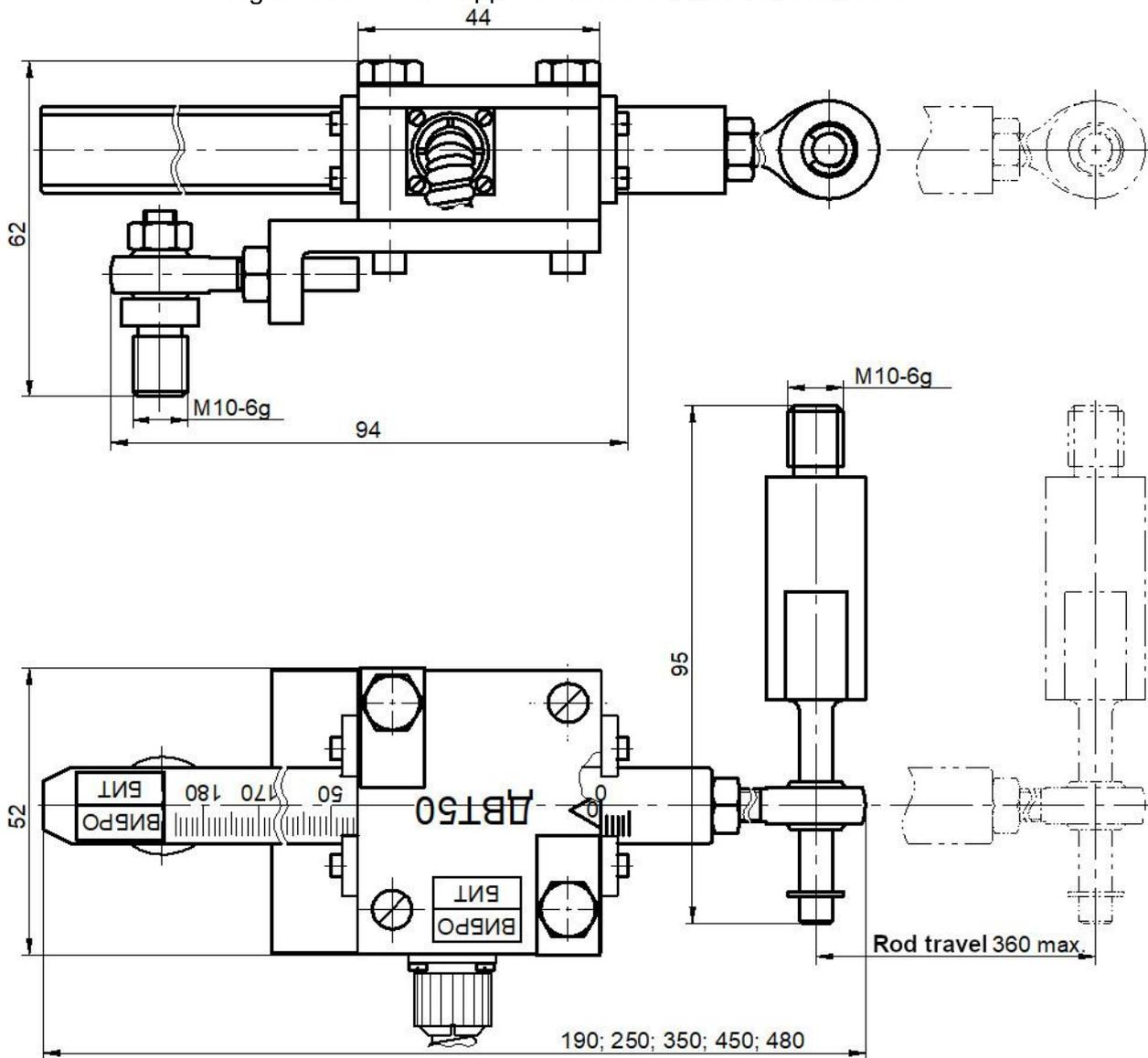
Figure C.10 – Sensor ДБТ50 with rod ВШПА.421412.060.04
