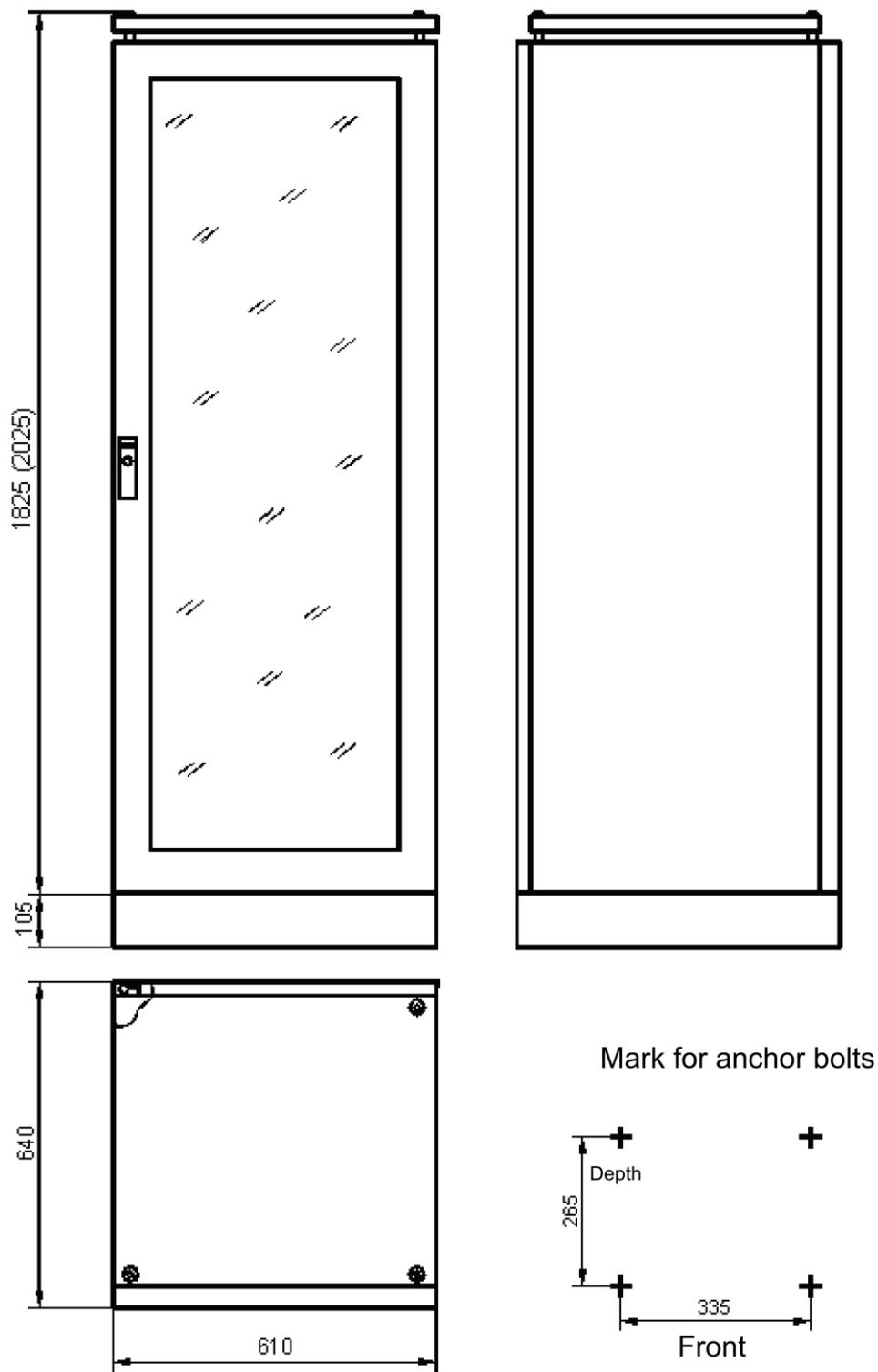
Anchor bolts M10 – (60±0.5) mm height above the concrete foundation.
