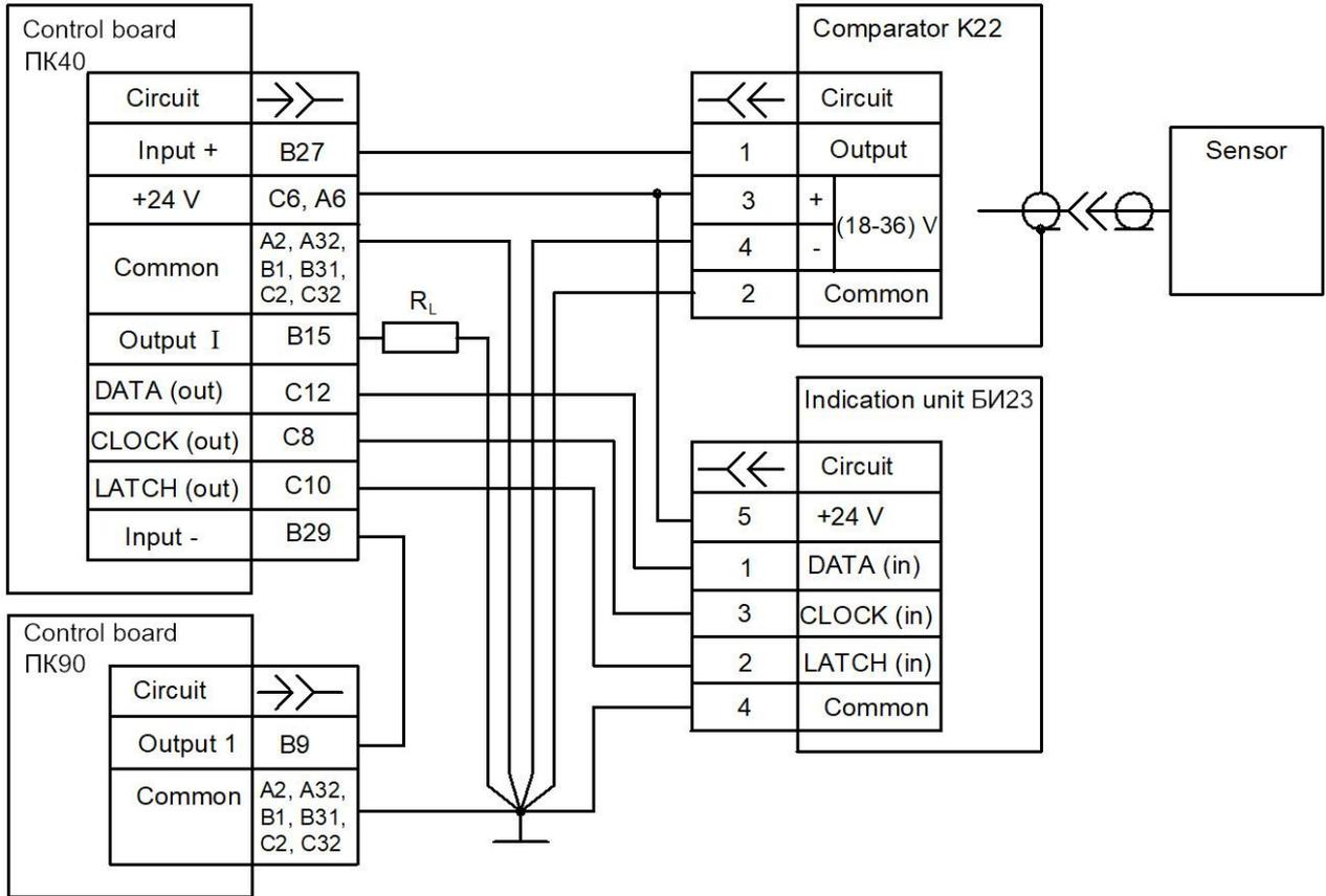
$R_L$  – unified signal load resistance.
