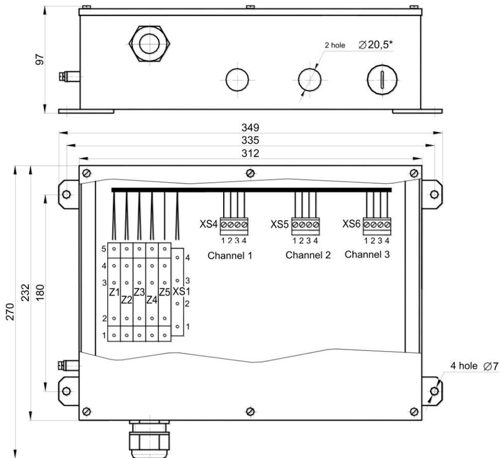
Figure C.36 – Transducer box КП25
