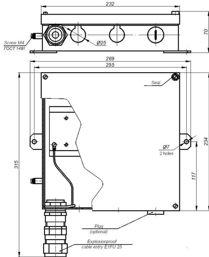
Figure C.35 – Transducer box КП23ПХ
