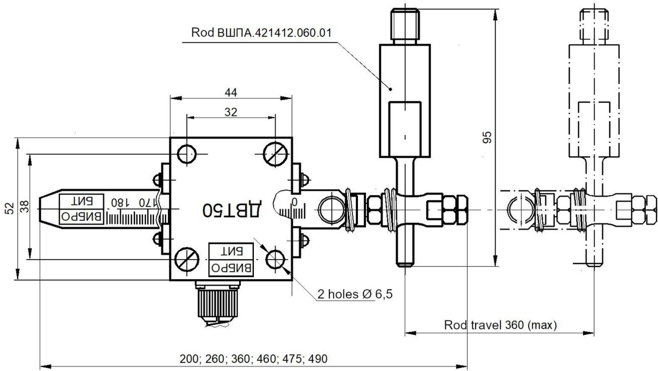
Figure C.9 – Sensor ДБТ50 with rod ВШПА.421412.060.01
