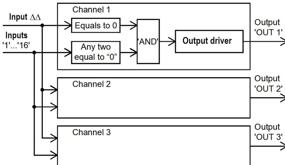
Figure 5 – block diagram of board ПК74
