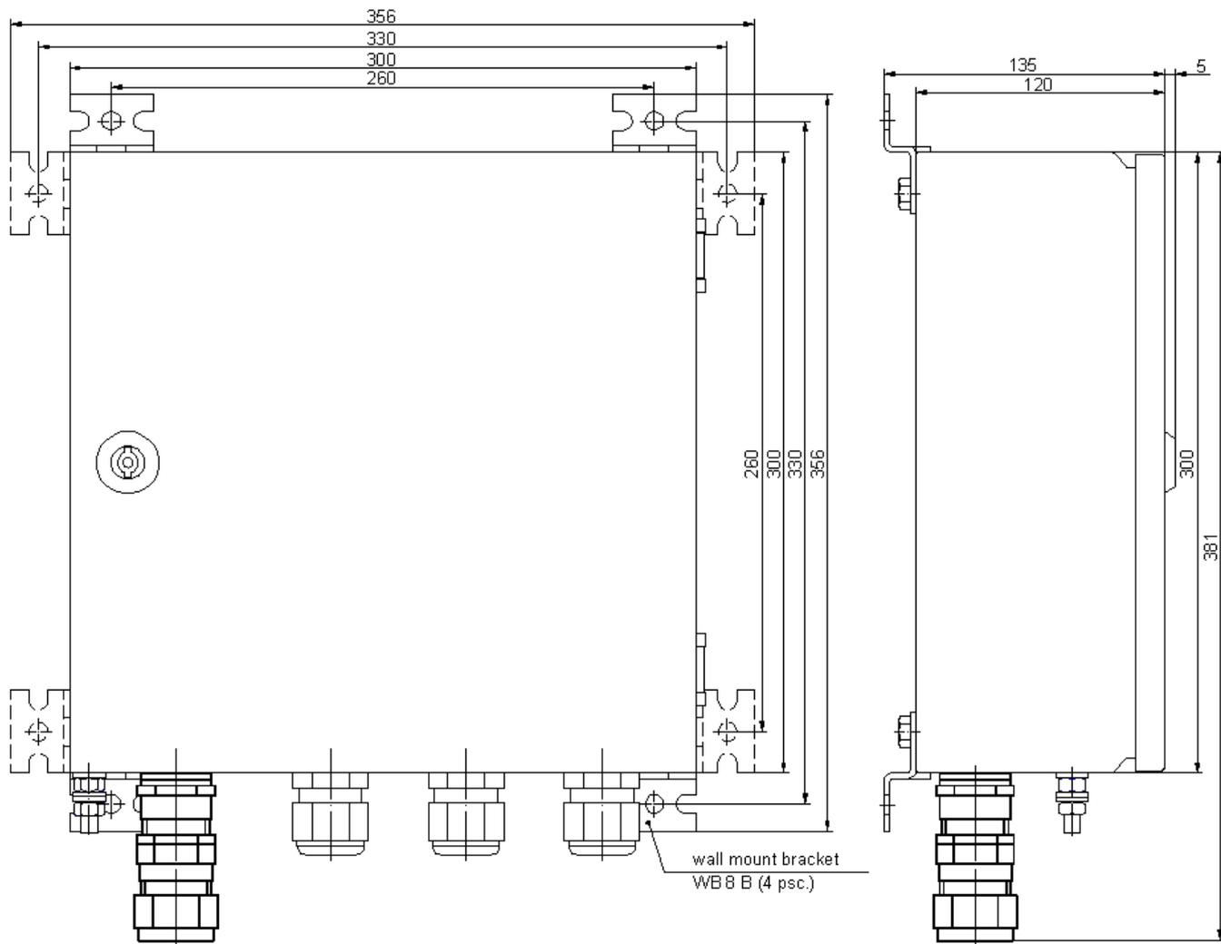
Figure C.47 – Transducer box КП23Х-Пр
