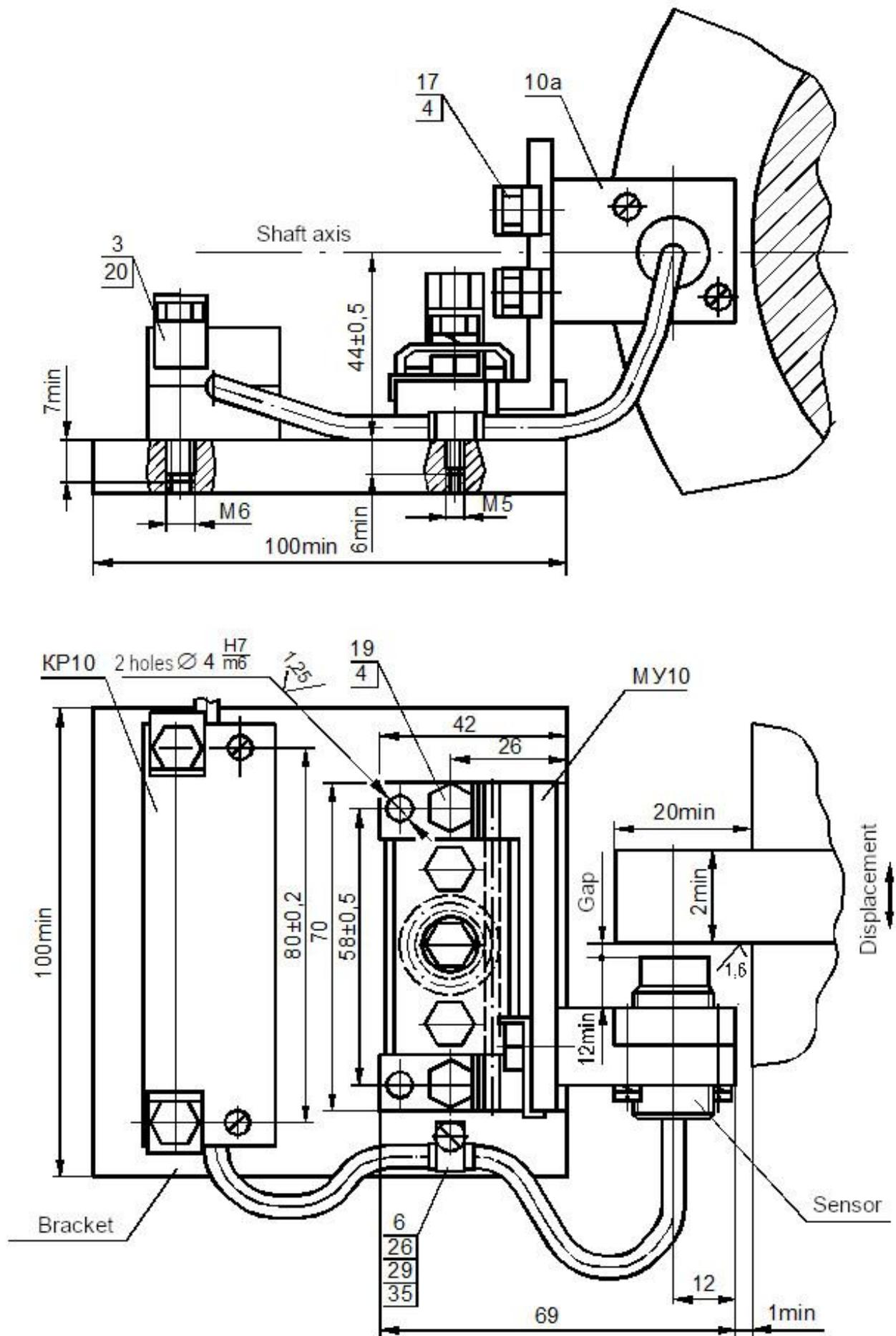
Figure K.5 - Installation of the sensor basing on ВШПА.421412.000.15.
