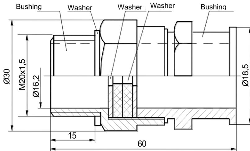
Figure C.28 – Feedthrough M20
