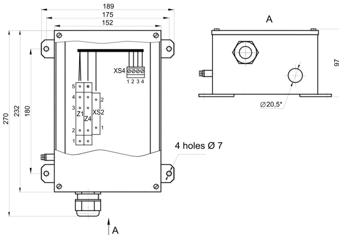
Figure C.37 – Transducer box КП15
