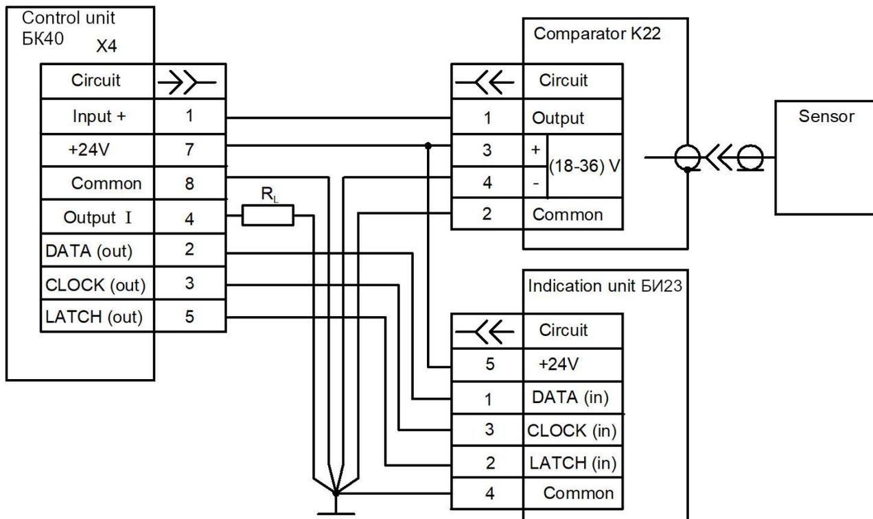
$R_L$  – unified signal load resistance
