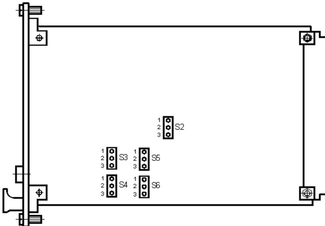
Position of jumpers determining eight inputs for 'M' and 'M1' memory registers
