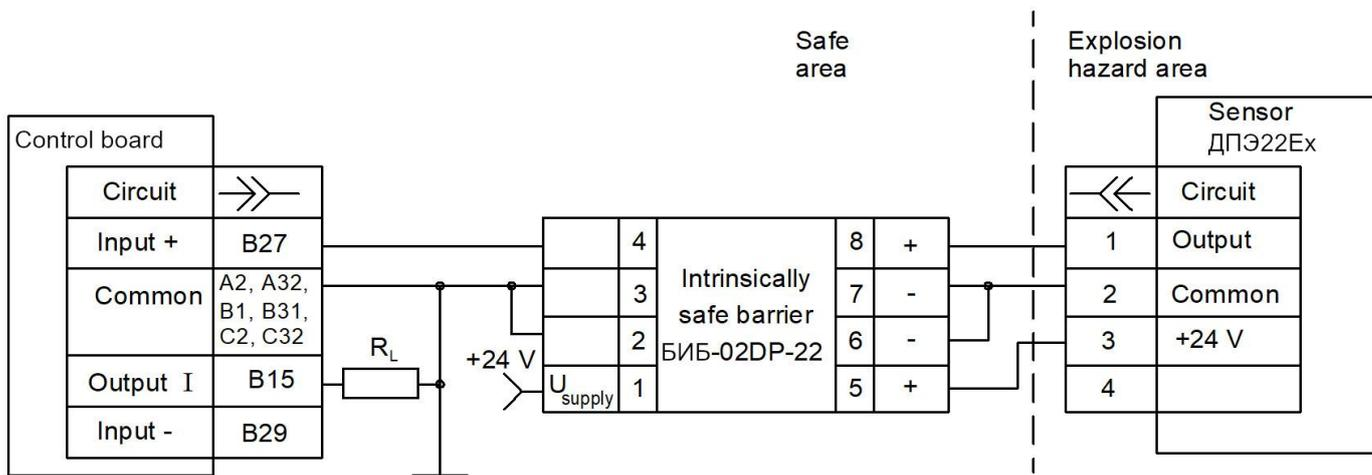
$R_L$  – unified signal load resistance.
