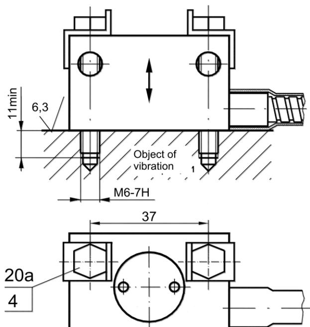
Figure K.18 – Setpoint of sensors ДПЭ22П, ДПЭ23П
