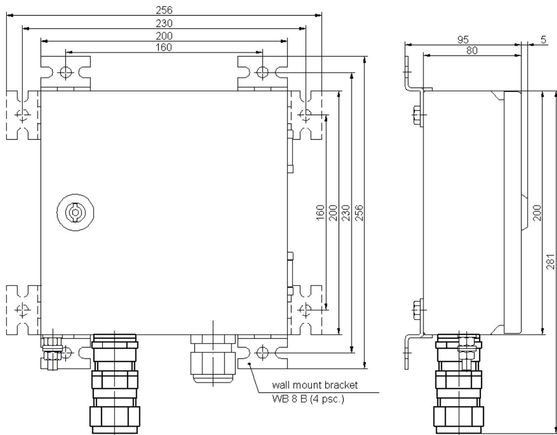
Figure C.45 – Transducer box КП13Х-Пр1
