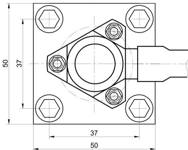
Figure K.22 – Installation of sensors ДПЭ22МВ, ДПЭ22МВТ, ДПЭ23МВ, ДПЭ23МВТ with insulated metal hose
