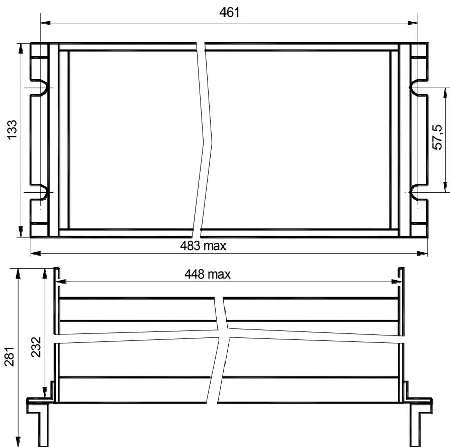
Opening for installation of framework 134x449 mm (max)
