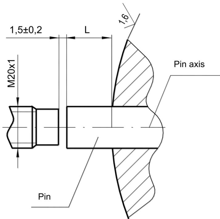
L – Pin protrusion distance
