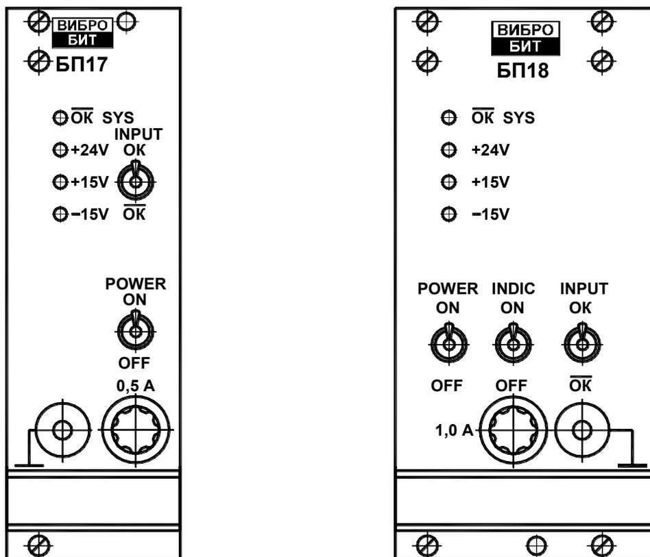
Figure B.3 – Power supply units БП
