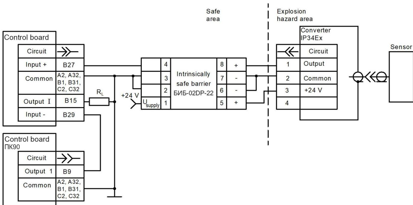
$R_L$  – unified signal load resistance.
