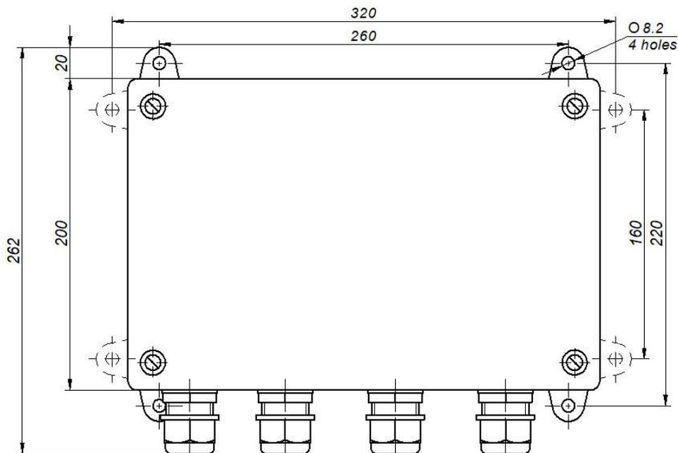
Figure C.42 – Transducer box КП23BP
