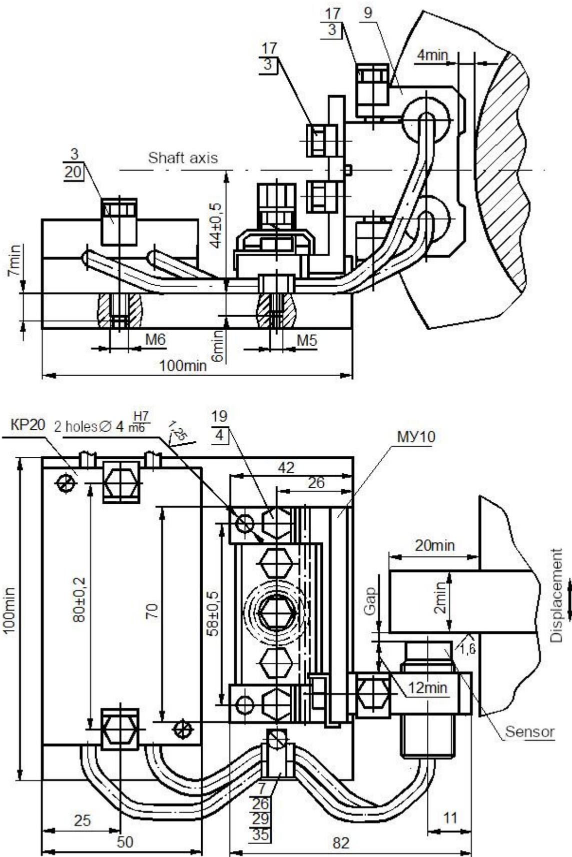
Figure K.6 - Installation of the sensor basing on ВШПА.421412.000.28.
