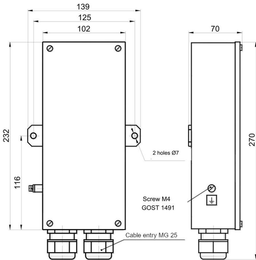
Figure C.38 – Transducer box КП13, КП13K
