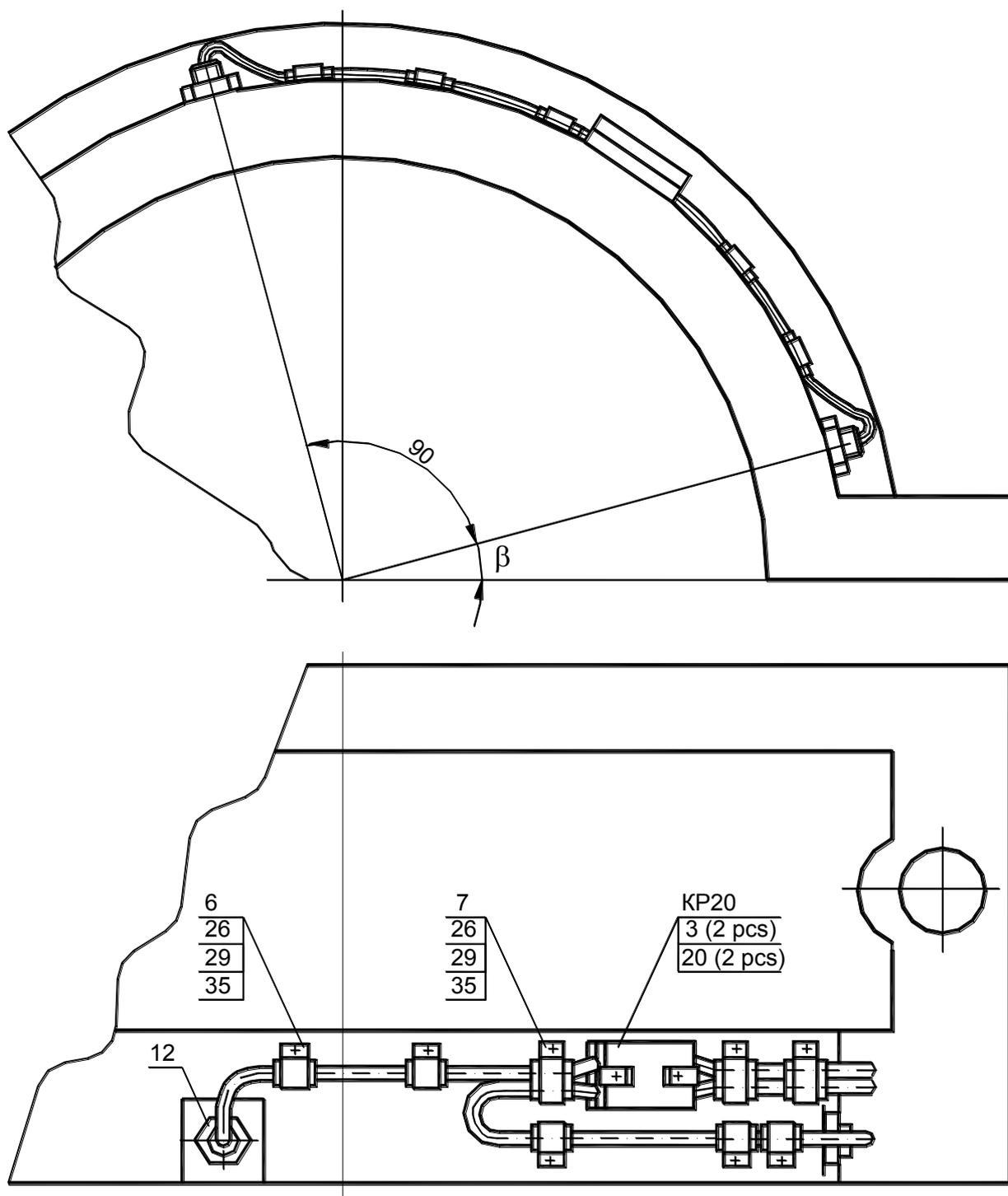
Cabling from the rotor side to the coupling side depends on the bearing design.
