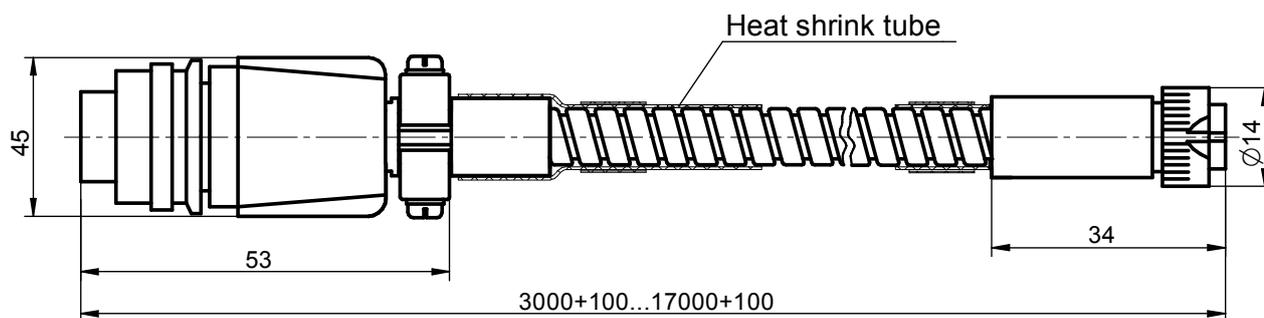
Figure C. 27 – Connection cable KC24
