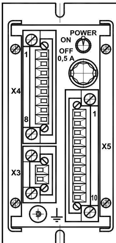
Figure B.7 – Arrangement of connectors at БК unit back panel
