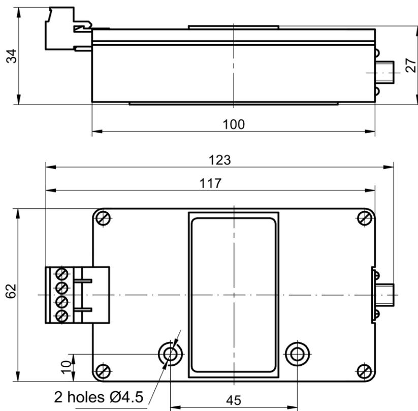
Figure C.25 – Converters ИП24, ИП42, ИП43, ИП44
