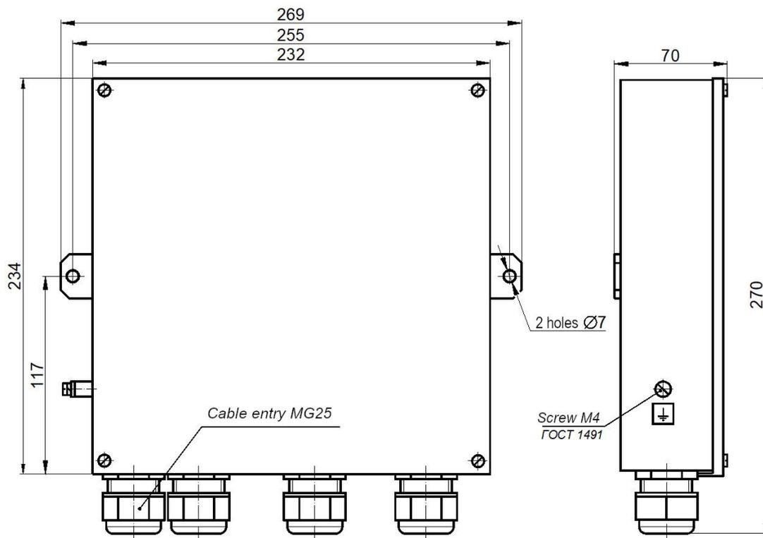
Figure C.32 – Transducer box KP23B
