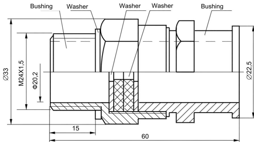
Figure C.29 – Feedthrough M24
