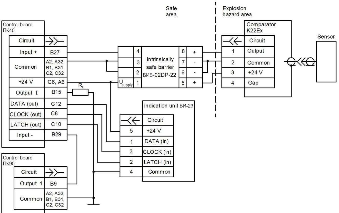
$R_L$  – unified signal load resistance
