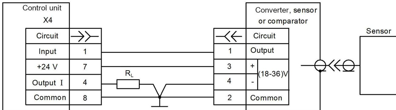
$R_L$  – unified signal load resistance.
