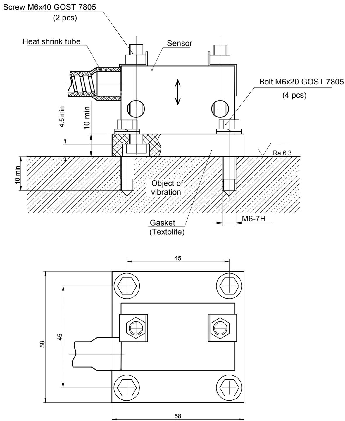
Figure K.23 – Installation of sensors ДПЭ22П, ДПЭ23П with insulated metal hose
