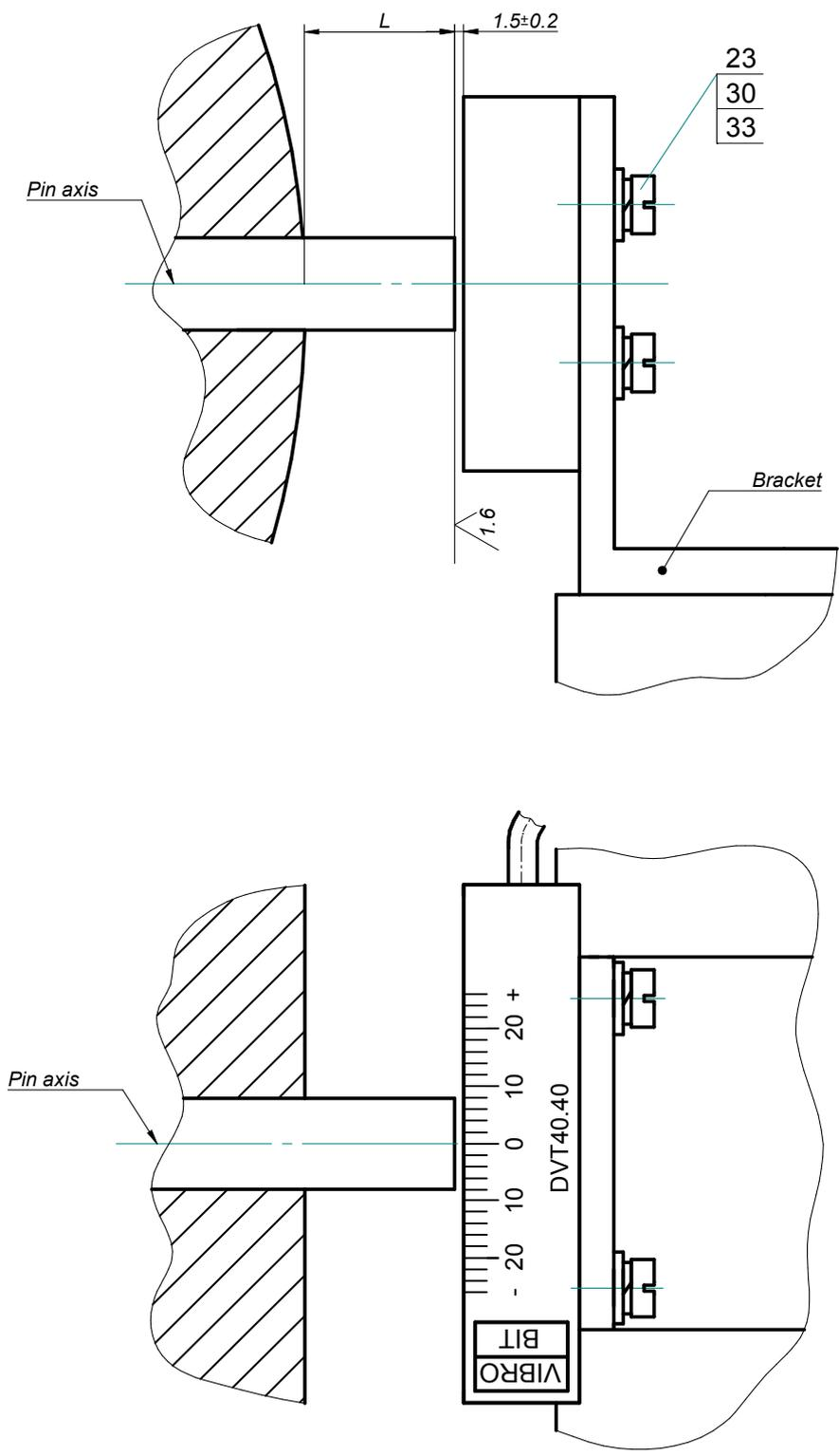
L – Pin protrusion distance ( $L_{\min}=3$  mm)
