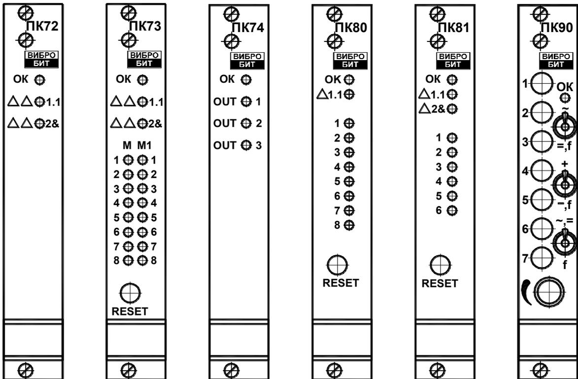
Figure B.2 – Control boards ПК
