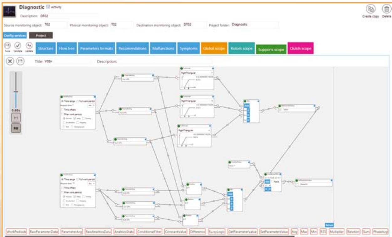
Upon units' connection between themselves, input and output parameters setup of every unit, diagnostic algorithm adapts to the extent possible to the specific diagnosed object.
