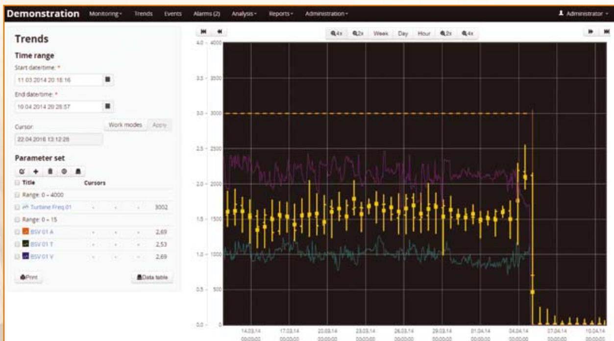
Parameters presentation on graph as candles enables to analyze parameter measured data over large time period.
